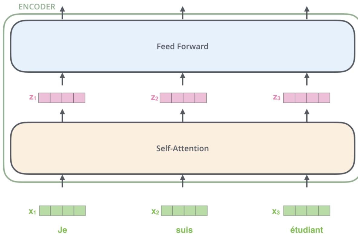
A key property is that each input element  $x_i$  follows an independent path in the network. There are **dependencies** between these paths in the **self-attention layer**. The **feed-forward layer** does not have any dependencies.
