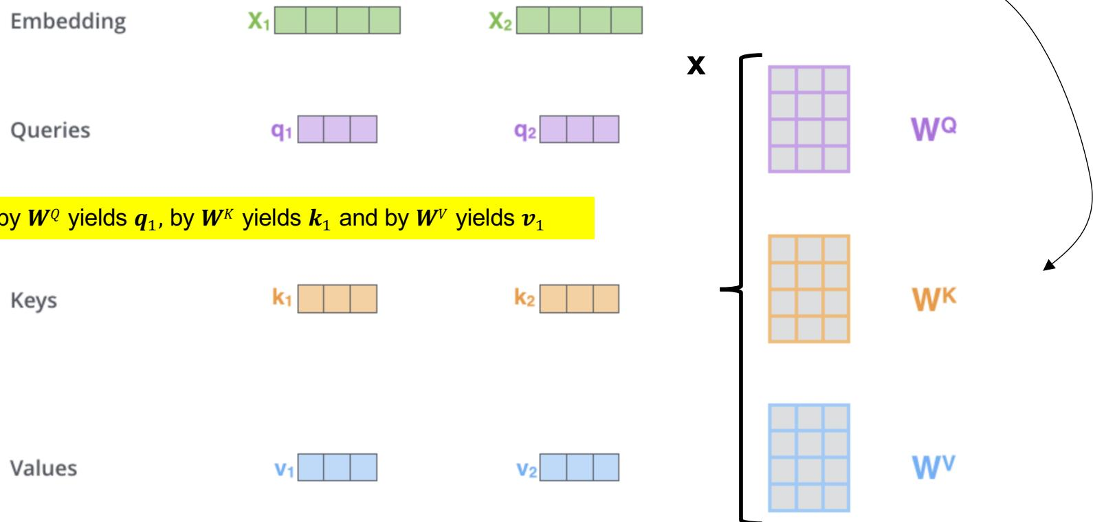
Typically, the dimensionality of the query, key and value vectors is smaller than the dimensionality of the embedding (e.g.,  $64 << 512$ )
