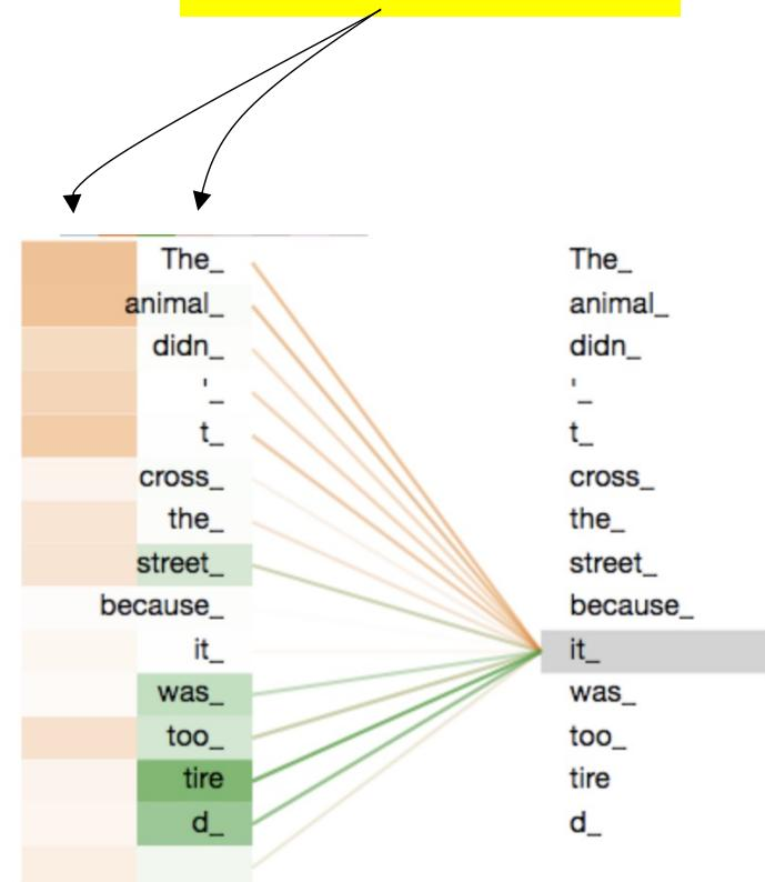
❤️ This is the “heart” of the Attention mechanism. To **replace** a representation of the input element by a **linear combination** of the other elements in the space, depending on the similarity/importance of each one with respect to the input. ❤️
