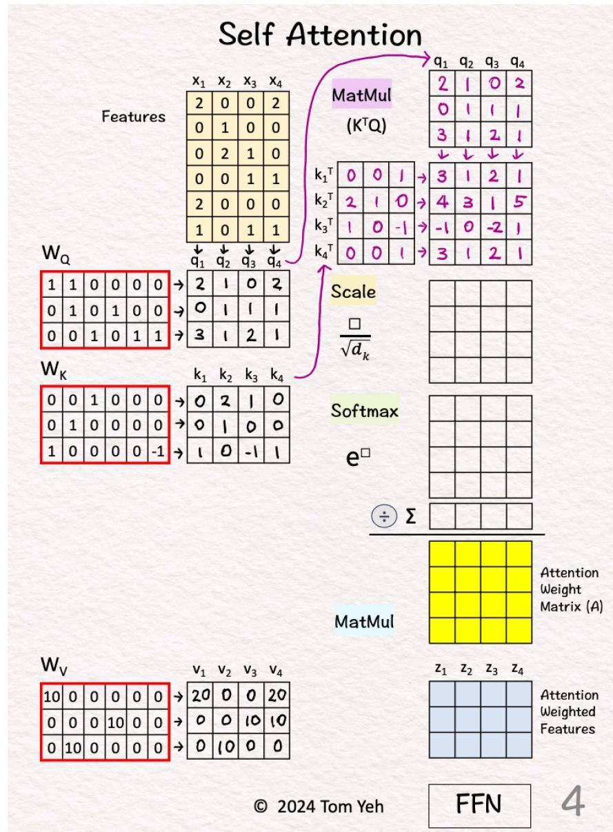
**Step 3.** Scale each element by the square root of  $d_k$ , which is the dimension of key vectors ( $d_k=3$ ).
