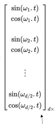
The positional vector contains pairs of sines and cosines of different frequencies. It is added to the embeddings. ("t" is the position of the token in the context)
