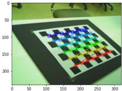
To calibrate the camera, in addition to the coordinates of the corners in each image, the threedimensional coordinates of the corners in the reference system of the scene should be given.
