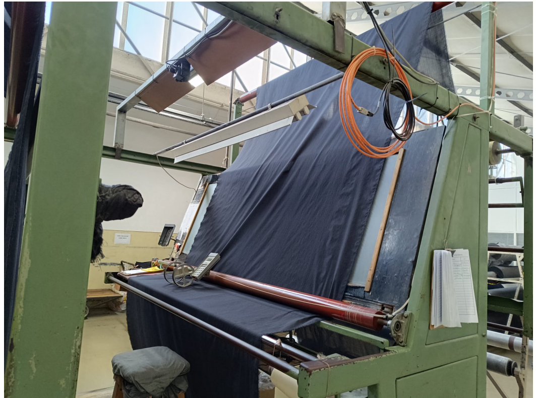
Figure 1. Typical final inspection stage, from a textile factory in Portugal. Factories in many countries have a workflow and equipment similar to this one.
