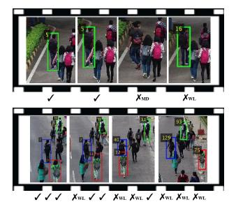
Fig. 7. Examples of sequences where the tracking methods faced difficulties, either missing the ground-truth targets at some point or producing a *fragmentation* that resulted in a wrong label assignment. *MD* stands for "missed detection" and *WL* represents "wrong label" assignment.
